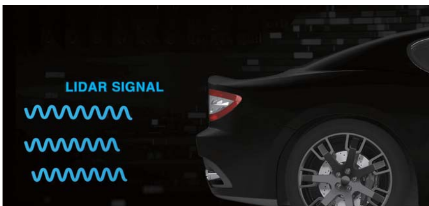
Conventional carbon black absorbs LiDAR near-infrared rays, reducing responsiveness.
